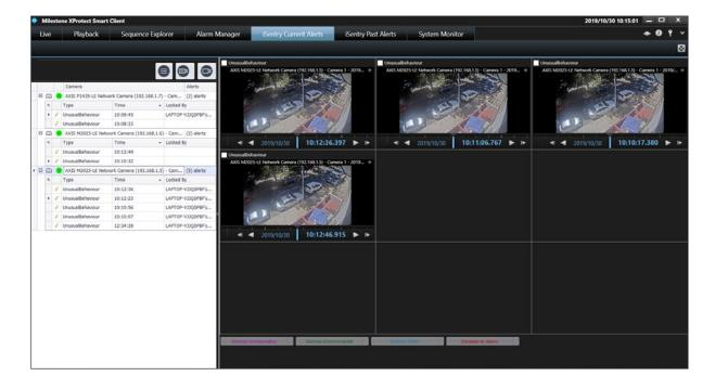
When a device (camera) is clicked, in the alert list (when cameras are visible), the multiple alert processing window is displayed. This window will simultaneously play the video for up to nine live alerts. It is up to the operator to confirm that each video has been inspected by checking the checkbox in the top right-hand corner of each video, where after the selected alerts can be processed simultaneously.
