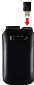
**Figure 3-4 Attaching Dongle**
