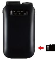
**Figure 3-3 Inserting Memory Card**
