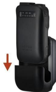
**Figure 3-5 Mounting External Battery**
