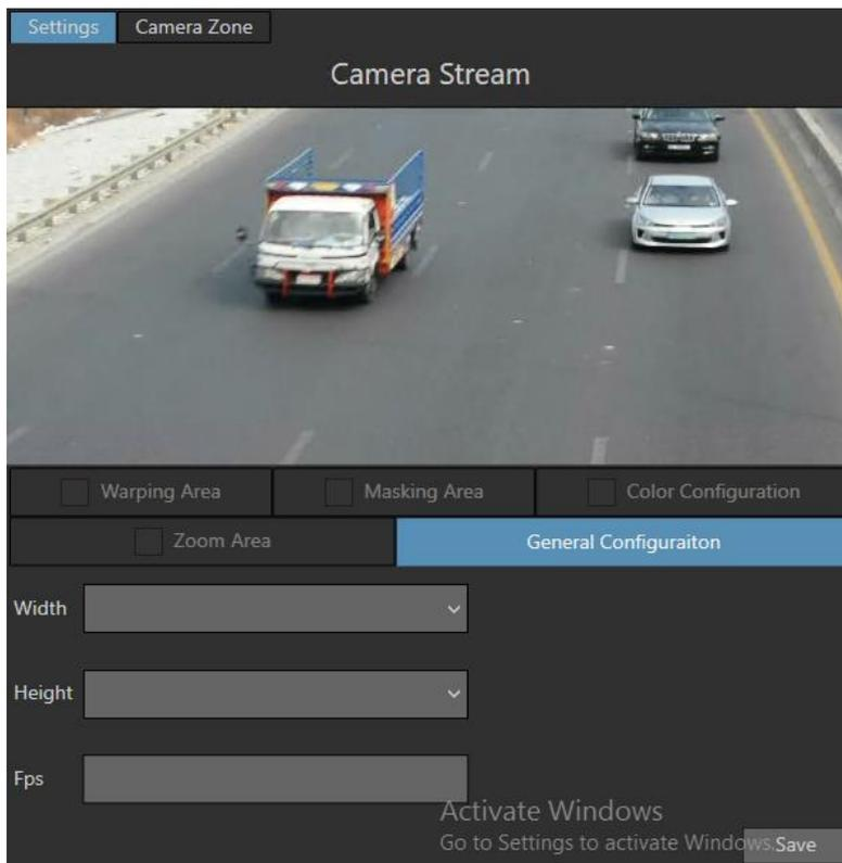
The window above is used to adjust the stream size: height, width and Fps (frame per second)
