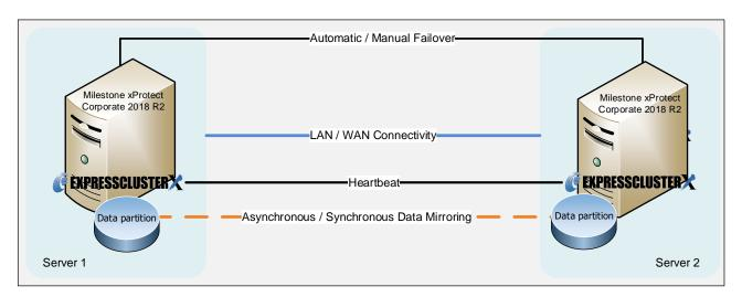
Configuration to cluster Milestone xProtect using NEC EXPRESSCLUSTER X had to be performed on the systems. Therefore, all the required service of the Application and its database were configured as per EXPRESSCLUSTER X requirement considering no impact of functioning of the application and its database.
