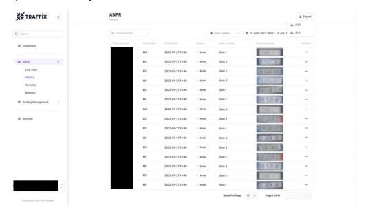
The **ALPR** (**Automatic License Plate Recognition**) **History** feature in Traffix provides a detailed log of detected vehicles, including license plate numbers, nationalities, entry dates, lane info, and captured plate images. This feature enables efficient monitoring, tracking, and management of vehicle movements for enhanced security and traffic control.
