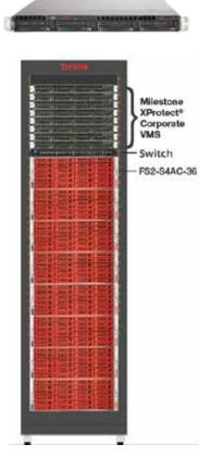
The customer specifically required a secure, scalable and cost-effective storage solution, so a single controller architecture was implemented. Tyrone recommended the Opslag FS2-S4AC-36 - a highly scalable solution offering storage capacity starting from a few TBs to PetaBytes.
