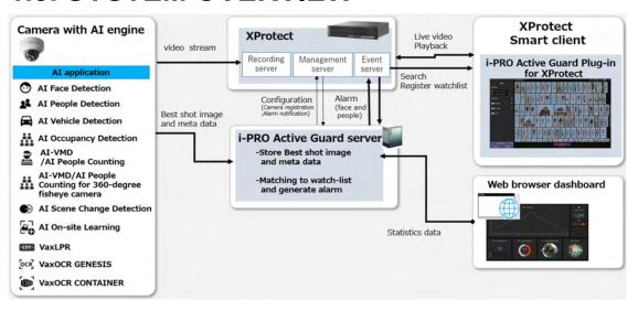
The AI application or AI function on i-PRO cameras transmit the video stream to XProtect and separately transmit Best shot images and metadata to the i-PRO Active Guard server.
