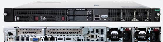
The 1U rack mountable server, powered by a redundant power supply and two Solid State Drives in redundant configuration ensures optimal performance. Two LAN ports allow the server to be connected to more than one corporate network enabling redundancy of the AV infrastructure and offering network flexibility and additional control.
