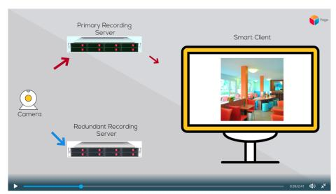
Figure 1: Dual Recording Concept
