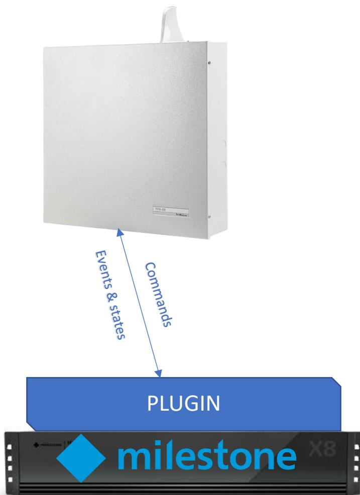
Due this architecture configuration, the panel needs to have the ESP-LAN module for the TCP/IP communication with the Plugin.
