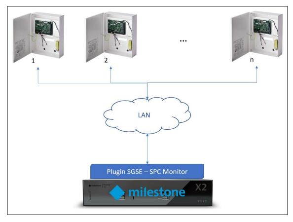
Through the Ethernet network, the plugin gets ready to accept connections from SPC intrusion panels. The SPC intrusion panel must be configured to communicate with the plugin as an ATP (Alarm Transmission Path) in an ATS (Alarm Transmission System). The basic panel configuration needed to work with this plugin will be described later in this document.
