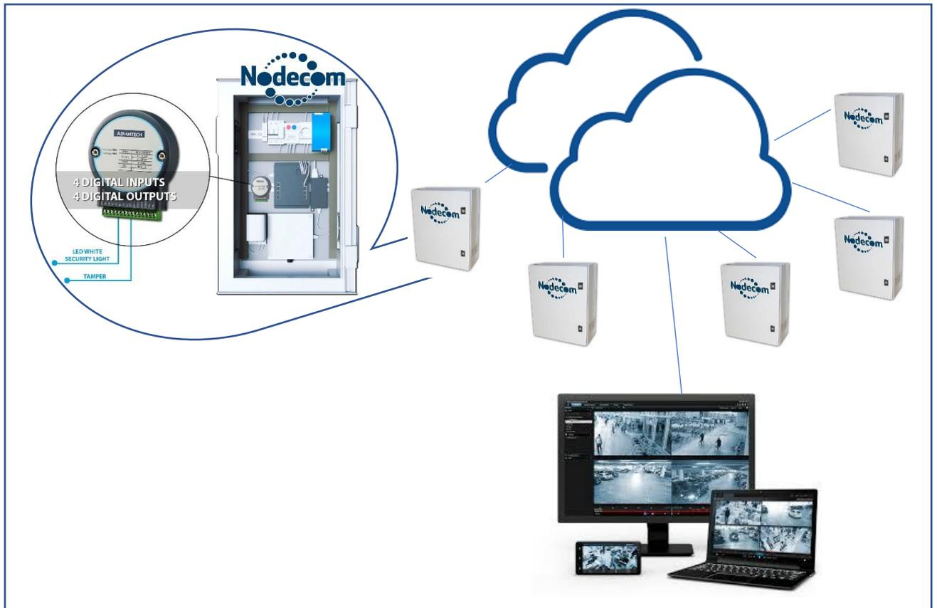
Through the Ethernet network, the plugin establishes communication with configured devices (Nodecom® cabinets).
