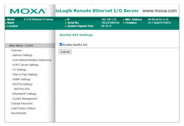
IMPORTANT: In the case of the Moxa E2210 device, it isn't possible to activate the RESTful API, since it doesn't have it. The plugin will communicate with the device through CGI commands.
