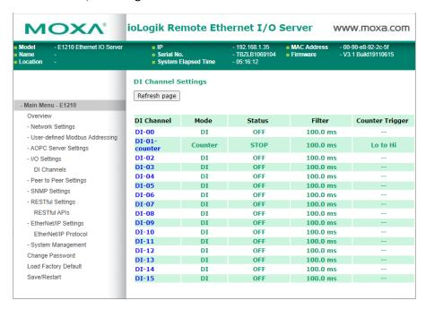
From this page you can click on any of the blue names of the channels and change operation mode to "DI".
