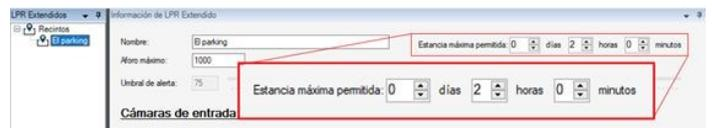
Thus, when a vehicle leaves the area, the system will calculate the length of time the vehicle has been in the area, searching for the previous reading made by the Milestone LPR system through one of the entrance cameras to the area.
