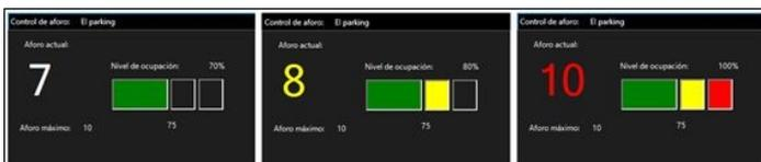
We can also set the occupancy level of the area manually in Smart Client, to correct any possible mismatches that may occur over time (undetected entry or exit, vehicles read twice, etc.)
